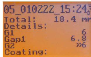
In the first row, the GlassBuddy Plus shows the position under which the measuring result is saved (here position 05; there are a total of 250 memory slots available). After this you can see the date and the time of the measurement.
