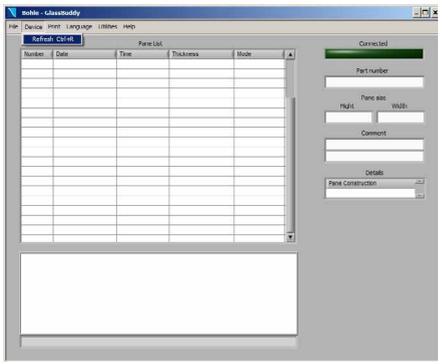
The programme is now connected to the GlassBuddy Plus. Once the connection has been established, the field "Connected" in the programme screen will turn light green. If this field does not turn light green, click on "Devices – Update" again.
