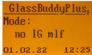
*Note: If you measure other glass types with this setting, this can lead to erroneous measuring results. Only fire protection gels from 1.4 mm - 3.2 mm are displayed as "Gel". Fire protection gels from 3.9 mm - 7.0 mm are displayed as "Layer". Build-ups deviating from this cannot be measured correctly.*
