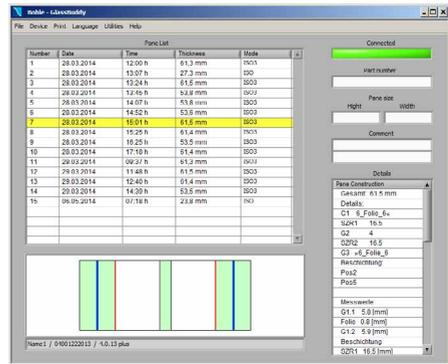
The graphic shows you the pane composition of the selected glass in the corresponding list. The results for glass (green), film (blue), fire protection gel (yellow) and layer (purple) are highlighted in different colours.
