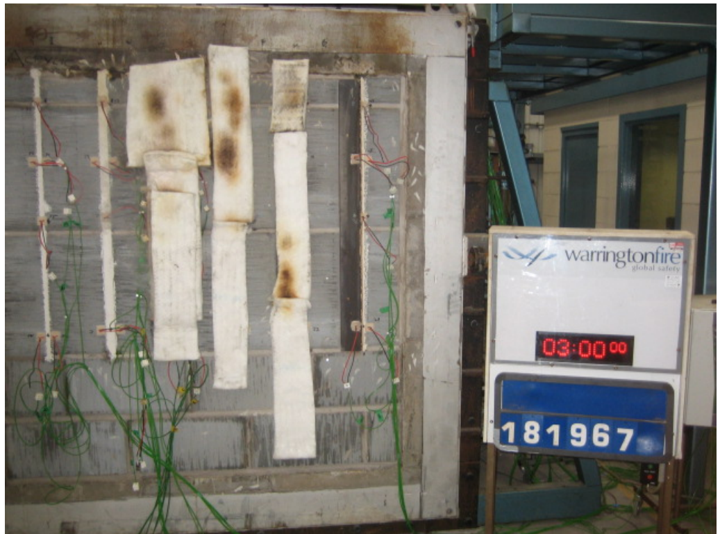
The unexposed face of the wall construction after 180 minutes of testing
