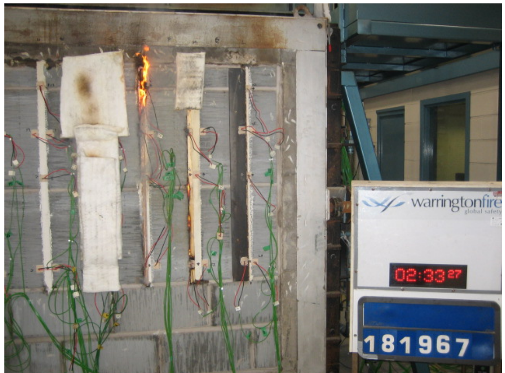
The unexposed face of the wall construction after 153 minutes of testing
