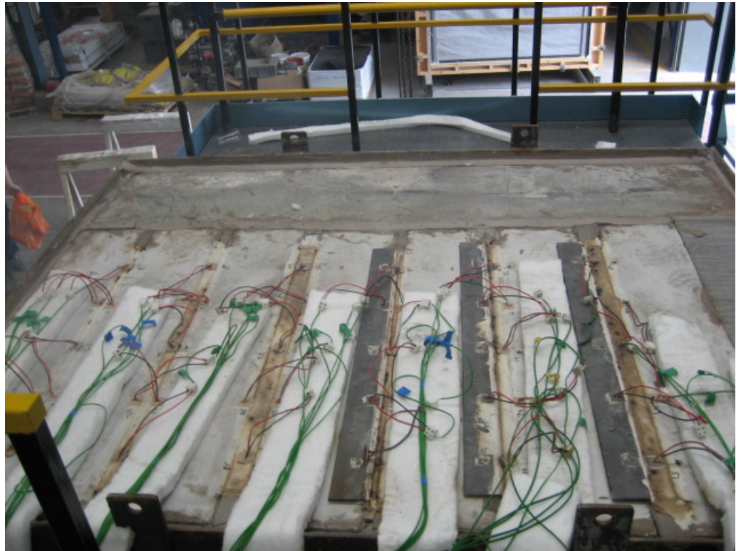
The unexposed face of the floor construction after 180 minutes of testing
