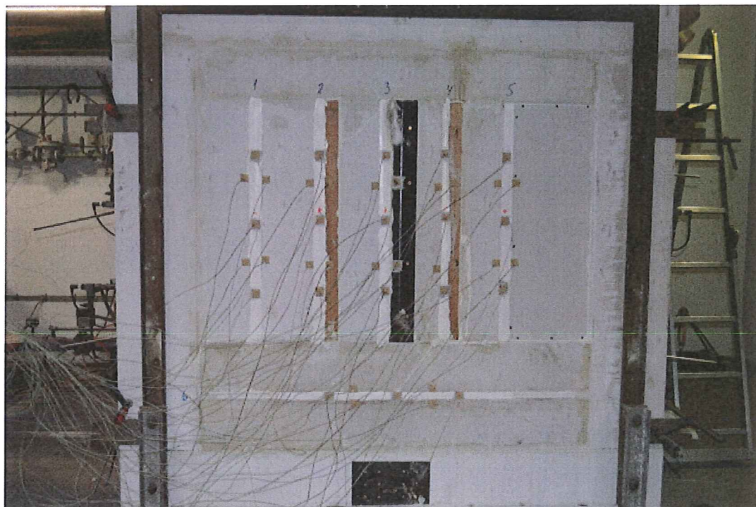
Photo No. 7 Unexposed side of test specimen after 60 minutes of testing
